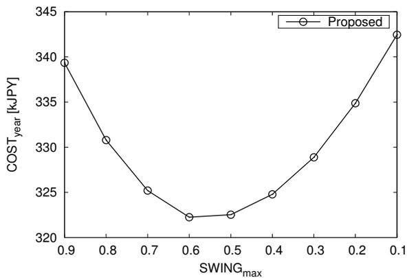
**Fig. 6** Total system cost of the proposed method with different upper bounds of the SOC swing
