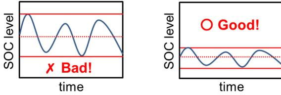
Fig. 1 Battery usage patterns
