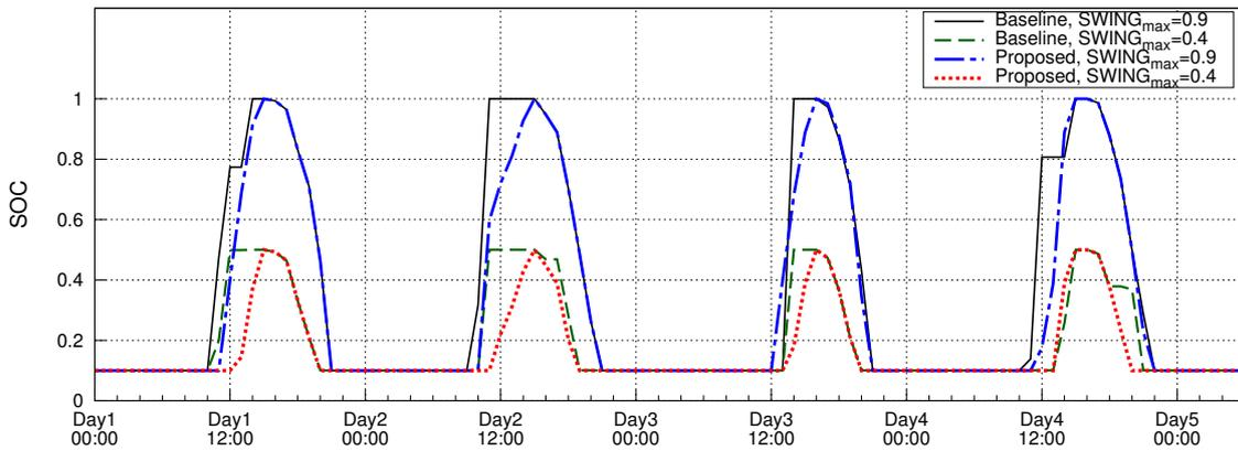
**Fig. 4** Batter SOC trace of Baseline and Proposed of cluster 1 for days in autumn with different  $SWING_{max}$
