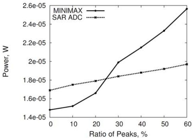
Figure 7: Measured Power Consumption of MINIMAX ADC.
