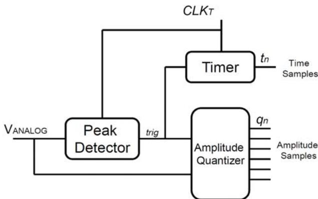
Figure 2: Structure of MINIMAX ADC.
